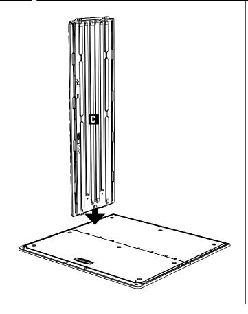
Using a screwdriver, punch out the screw holes on the top of Repeat Left Side (C) 2 places.
